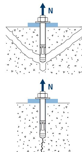
\*Concrete splitting design resistance must only be considered for non-cracked concrete.
